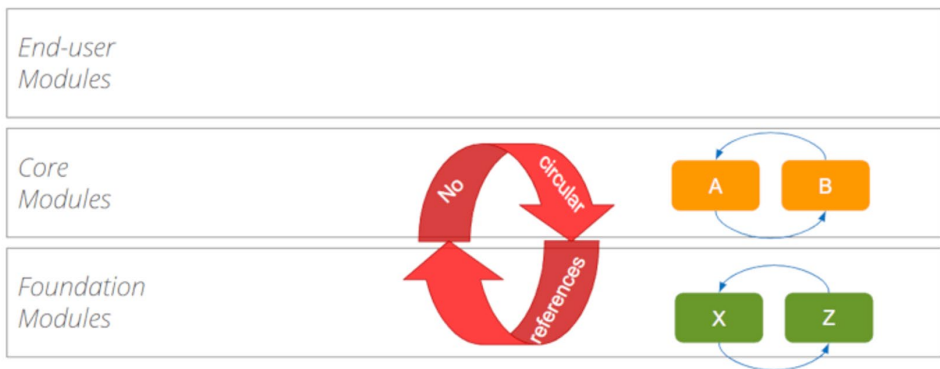
Fig. 9. Prevention of circular references between core and foundational modules
