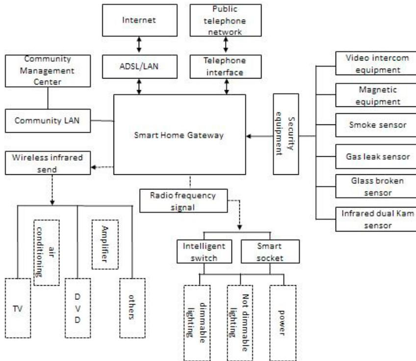
Figure 3.2. System structure
