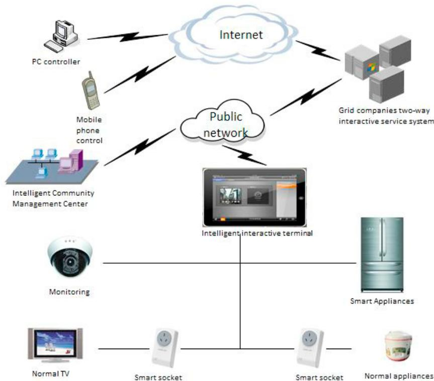
Figure 3.1. Structure of the system for electrical service of a smart home
