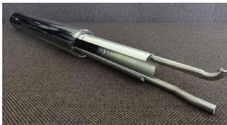
*Figure 3.3 Double glass tube (Dewar tube)*
