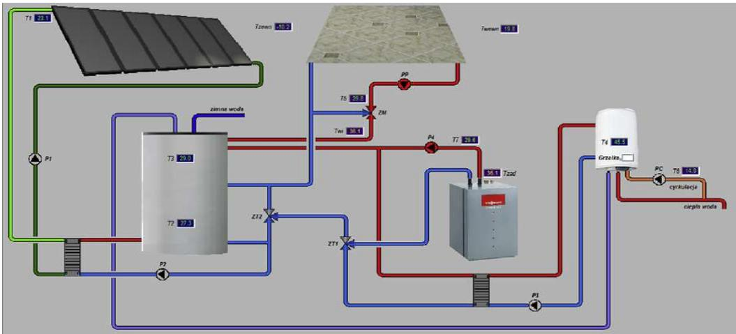
Figure 3.10 Solar heating system with a heat pump.
