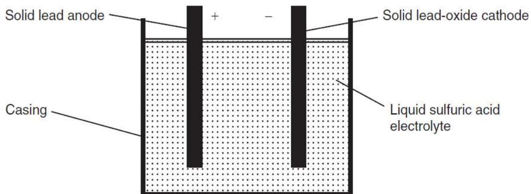
Figure 2.5. Schematic of a liquid-acid battery
