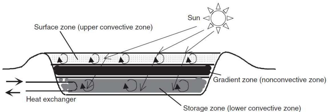
Figure 2.10 A cross-section representation of a typical salinity-gradient solar pond
