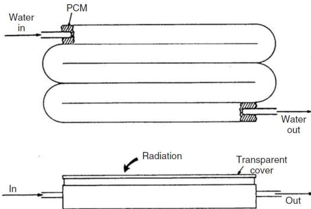
Figure 2.12 A solar TES pipe using a PCM
