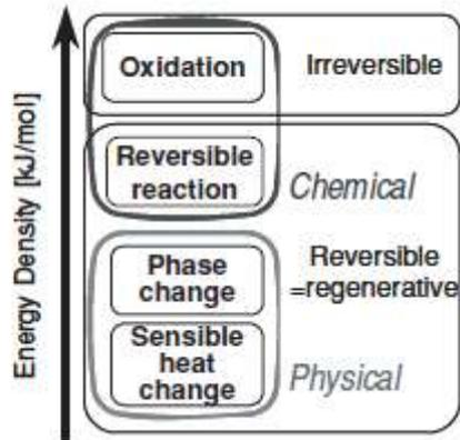
Figure 2.13 Energy density of physical and chemical changes
