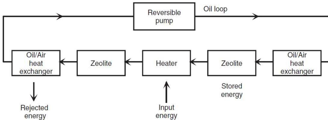
Figure 2.11 A process for using zeolites as a heat storage media
