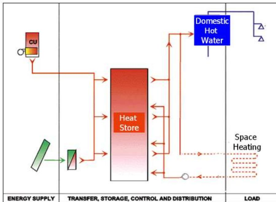
Figure 3.1 Solar system for domestic hot water and heating components
