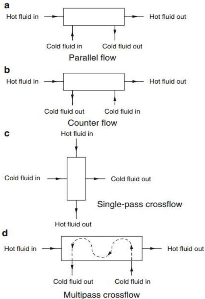
*Figure 3.4 Heat exchangers classification according to the flow path configuration*
