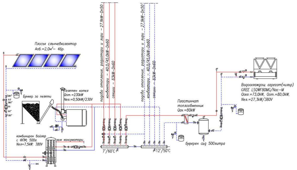
Figure 4.1 Combi-heating system detailed scheme
