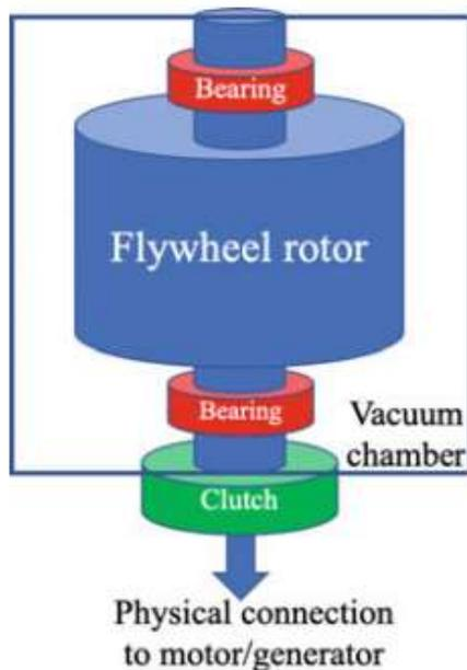
Figure 2.4. Main components of a flywheel energy storage system
