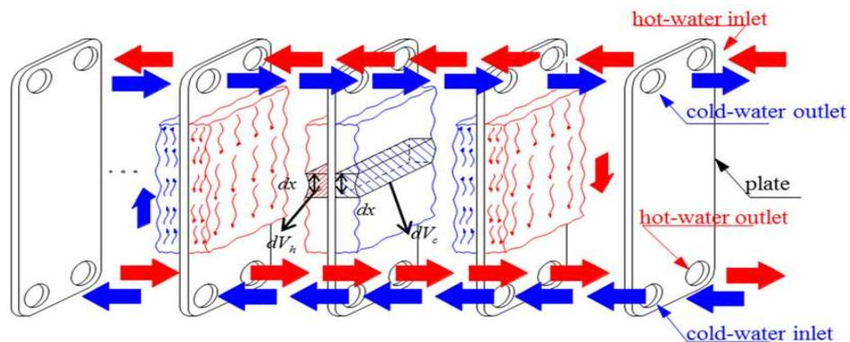
Figure 3.6 Plate heat exchanger
