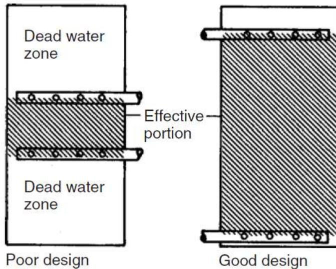
Φuzypa 2.7 Position of inlet and outlet for a thermally stratified TES tank
