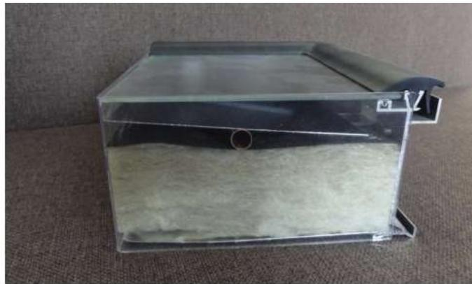
*Figure 3.2 A cross-section of a flat-plate liquid solar collector*
