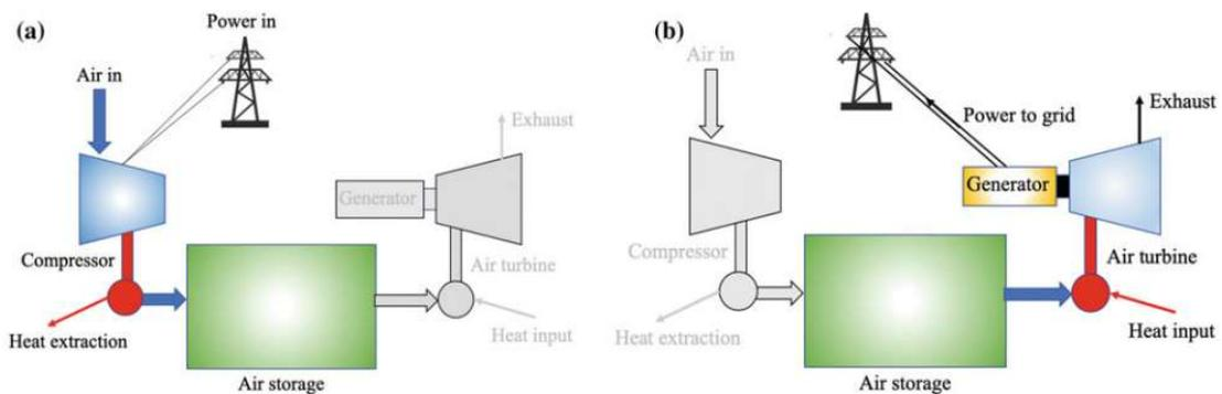
Figure 2.3 (a) Compressed-air system in charging mode; (b) discharging mode
