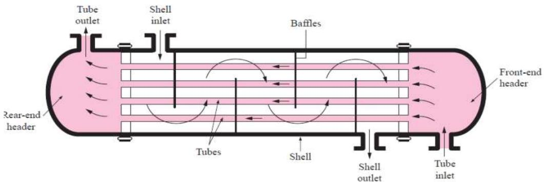
Figure 3.5 Shell and tube heat exchanger
