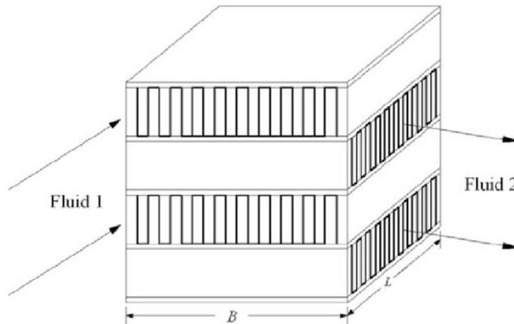
Figure 3.7 Plate-fin heat exchanger
