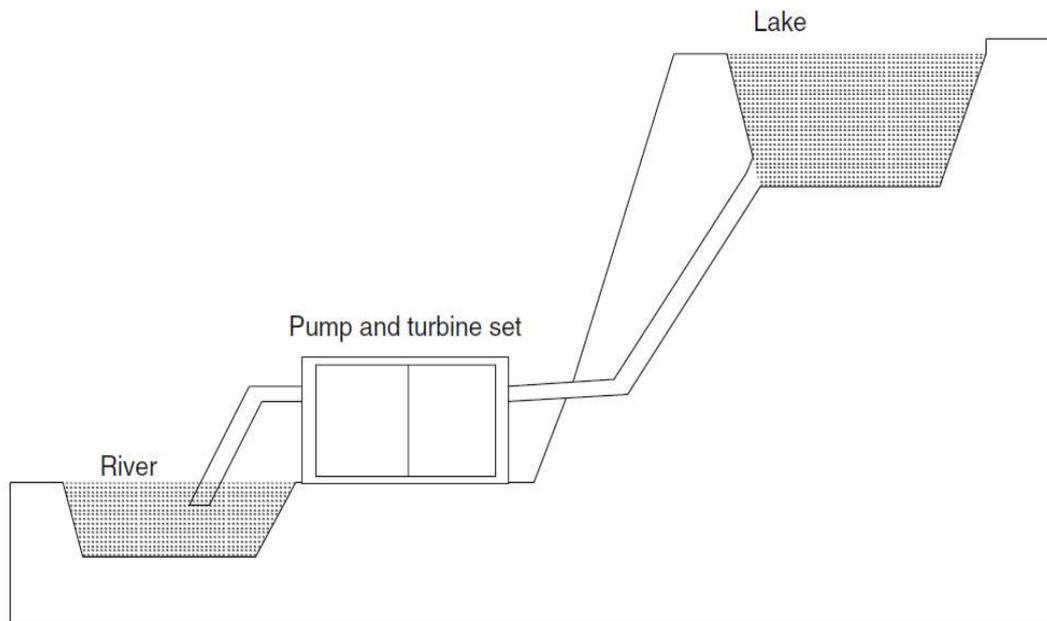
Figure 2.2 A pumped hydro storage plant
