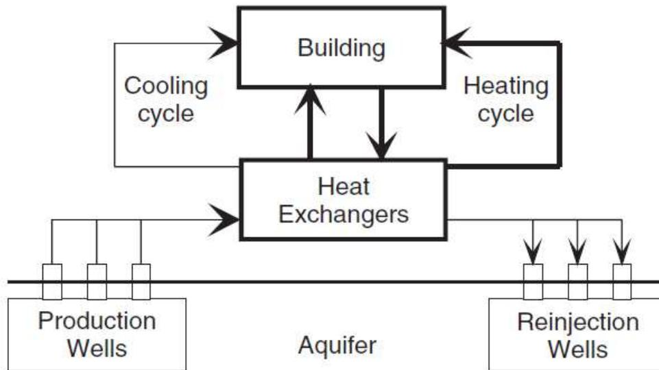
Figure 2.9 Schematic of the operation of an ATES system
