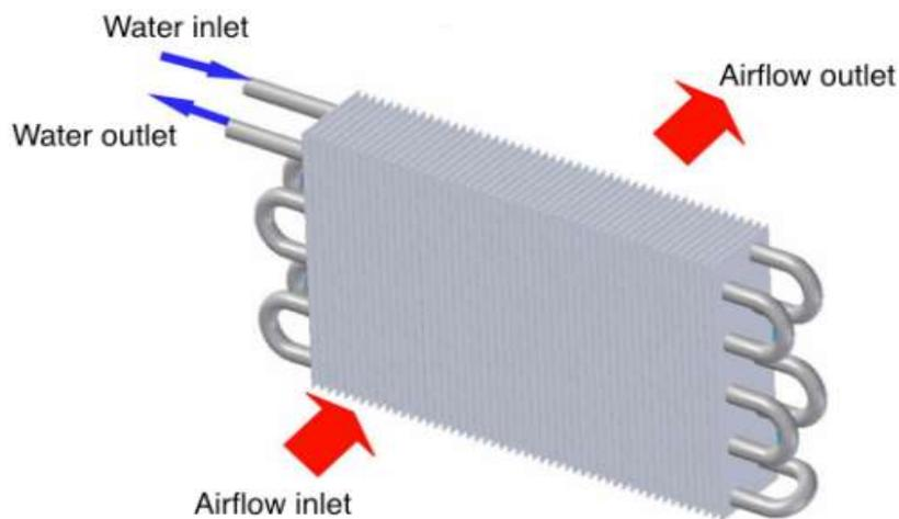
Figure 3.8 Flat finned tube heat exchanger
