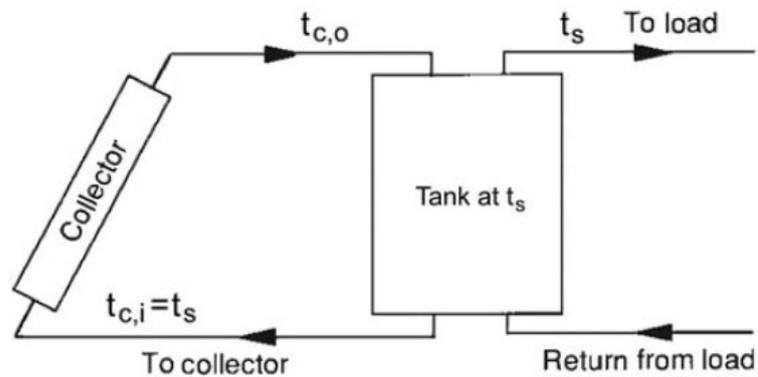
Figure 3.11 Solar system using a hot water storage tank
