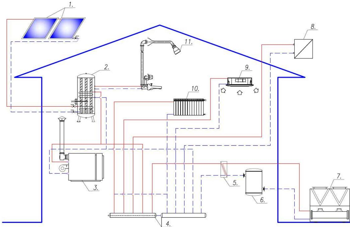
*Figure 3.13 Space heating system using PCM storage tank*
