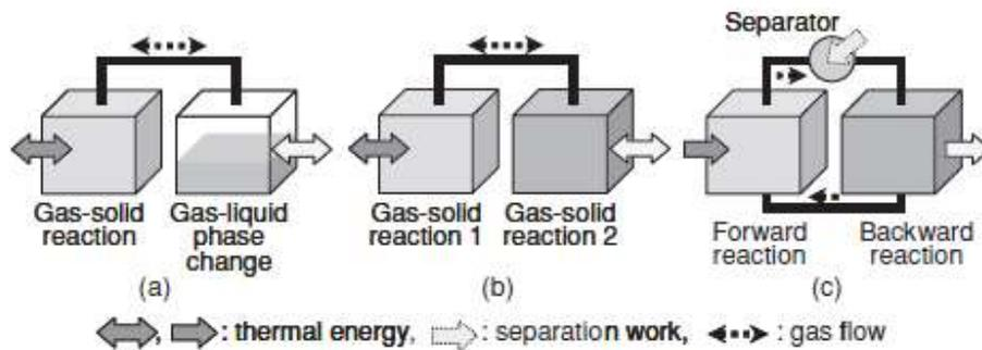
Figure 2.14 Types of chemical heat pumps; (a) reaction-phase change type, (b) reaction-reaction type, (c) reaction - continuous separation work type
