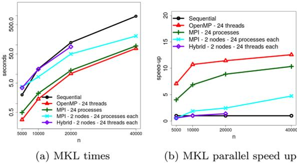
Figure 5: Parallel times and speed up with MKL.
