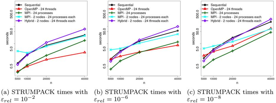
Figure 6: Times and parallel speed up for STRUMPACK.
