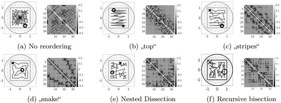
Figure 9: Reordering of the nodes in a square domain  $\Omega$  and the structure of the corresponding matrix. Dark gray lines represent the ordering of the nodes from the first (marked with “X”) and the last (marked with “O”).
