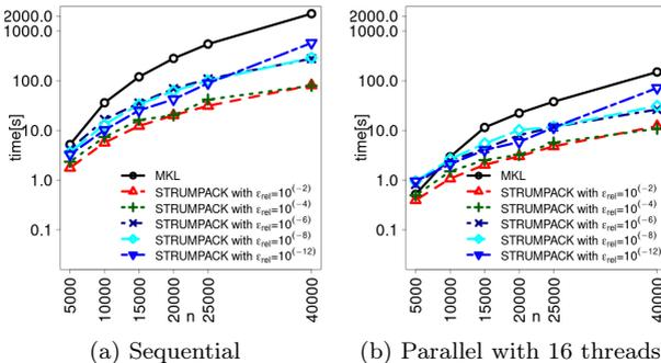
Figure 3: Performance of STRUMPACK in comparison with MKL
