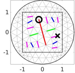
Figure 8: Reordering with nested dissection. “X” marks the first node, “O” marks the last.
