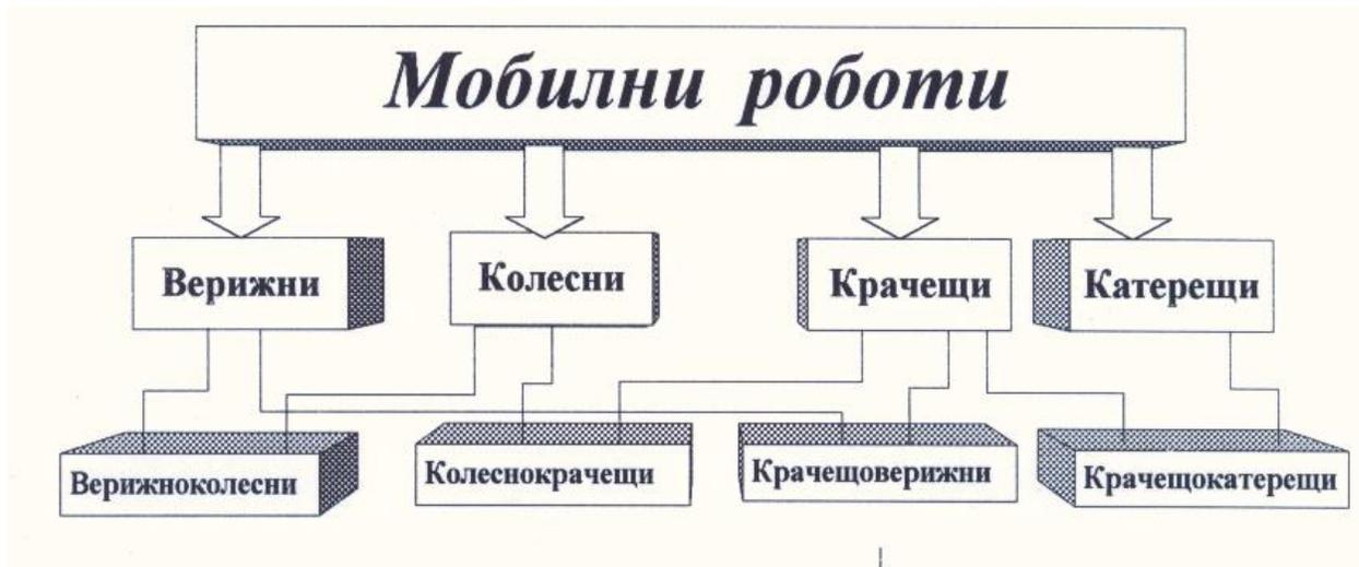
Fig. 1.1. Classification of mobile robots
