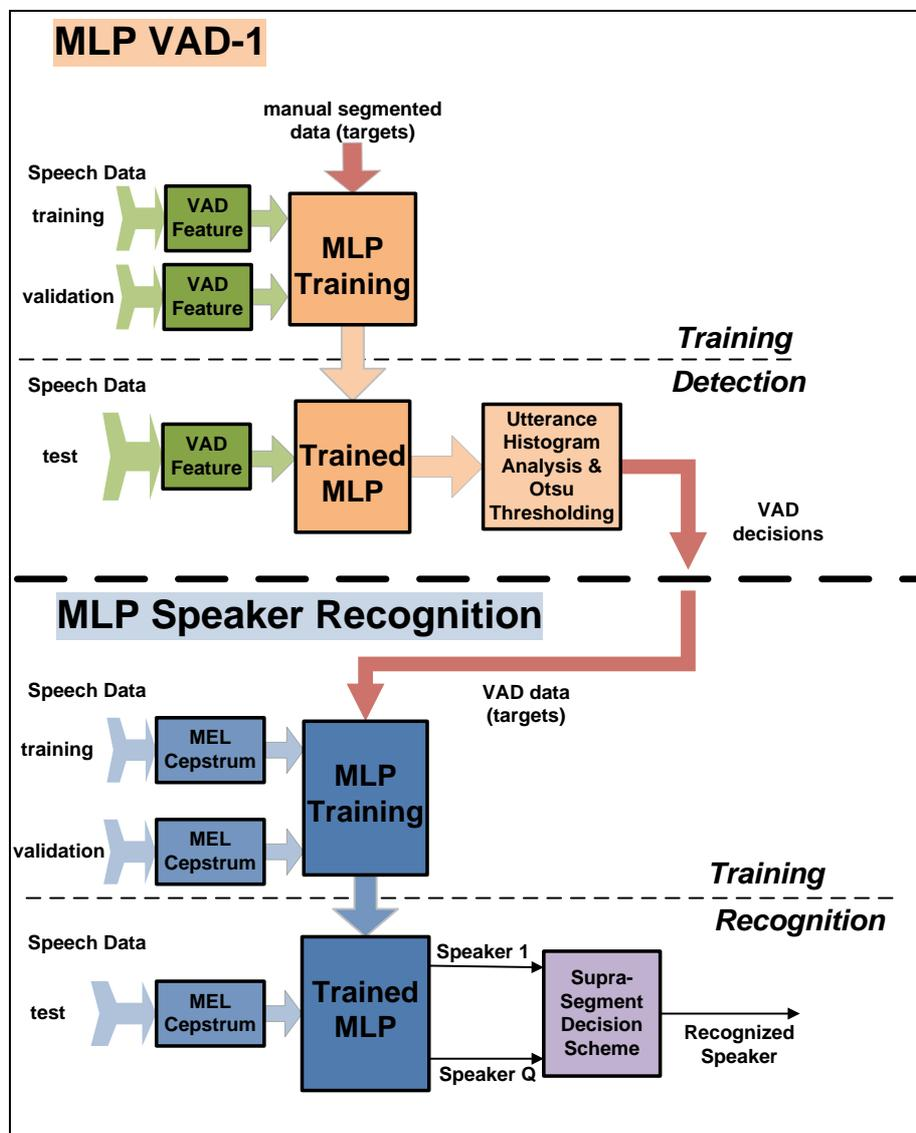
Fig.4.3. The block diagram of the MLP-based speaker identification system with details about VAD-1 algorithm.
