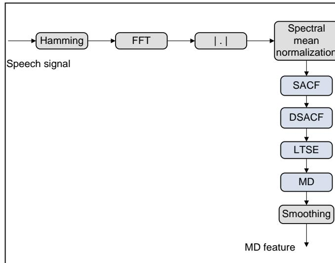
**Fig.2.10.** Block diagram of the algorithm for calculating of the MD feature.
