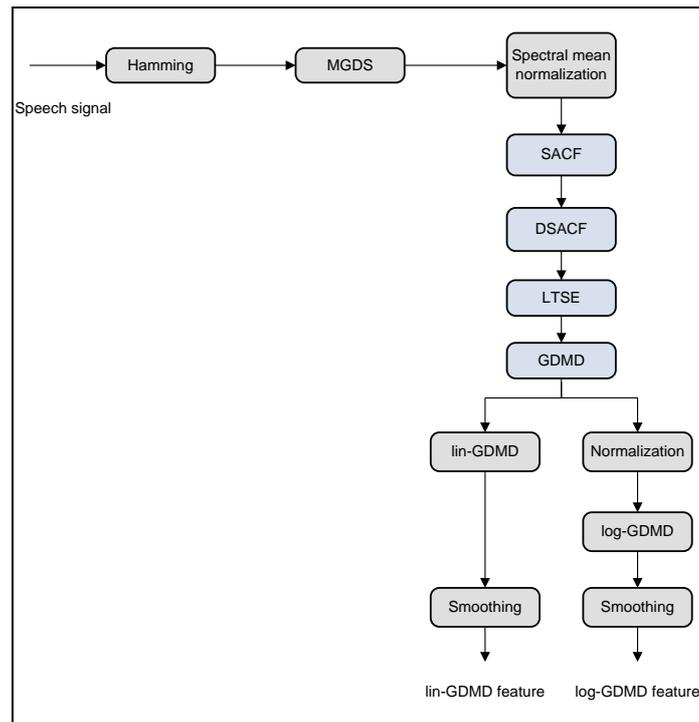
Fig. 2.12. Block diagram of the algorithm for the GDM features computing.
