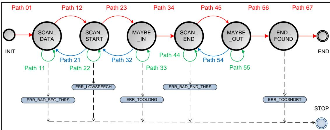
Fig.3.12. Finite state machine based decision logic diagram.
