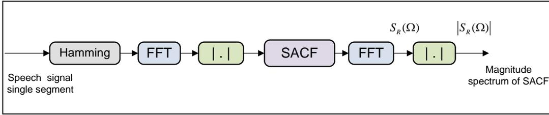
Fig.2.5. Block diagram of the algorithm for calculating of  $|S_R(\Omega)|$ .
