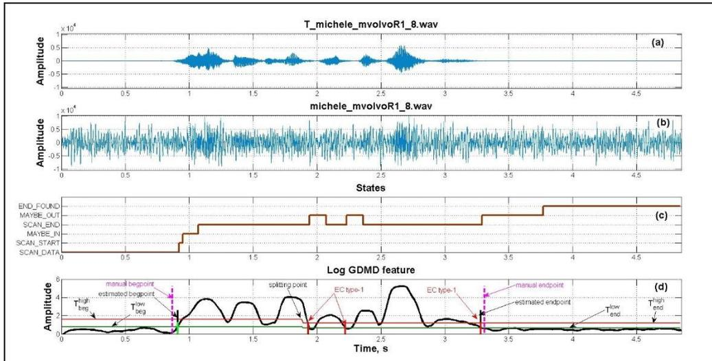
**Fig. 3.13.** Example from the SpEAR database: (a) clean signal; (b) noisy version; (c) the state transition timing diagram; (d) log-GDM feature contour with marked some details in temporal execution of the algorithm.
