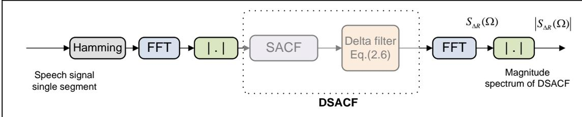
Fig.2.6. Block diagram of the algorithm for calculating of  $|S_{\Delta R}(\Omega)|$ .
