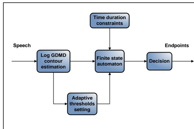
**Fig. 3.15.** The block diagram of the GDM-D-E detector.
