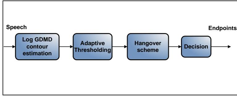
Fig. 3.17. The block diagram of the GDMD-H detector.
