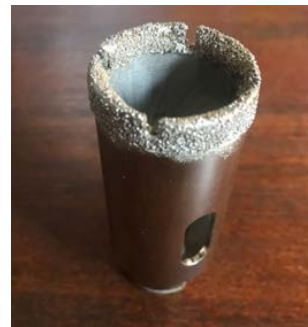
Fig. 22 Diamond tool for drilling
