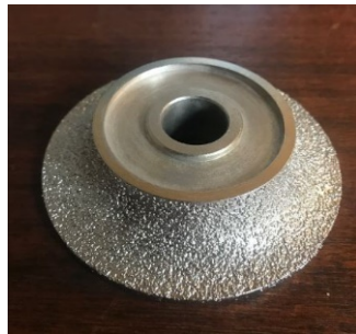
Fif. 21 Diamond tool for granite processing
