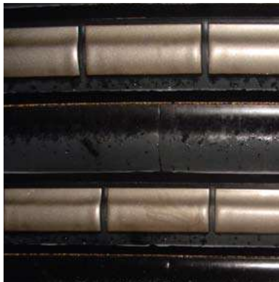
Above: Metal cap lining used near the grate end of a mill
