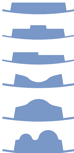
Various shell plate configurations, top to bottom: SFL, SCL, SSL, SSW, SDW and STW
