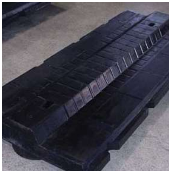
Above: Composite metal cap SFL shell lining
