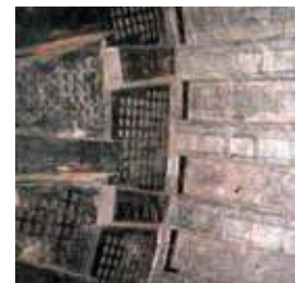
Above: Metal cap lining used near the grate end of a mill
