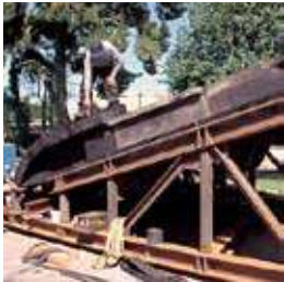
Above: Fit testing of pulp dischargers for large AG/SAG mill
