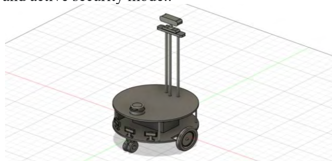
Fig. 63 Mobile robot-platform with mounted module for surveillance and security
