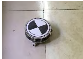
Fig. 6. The calibration plate on the intelligent agent
