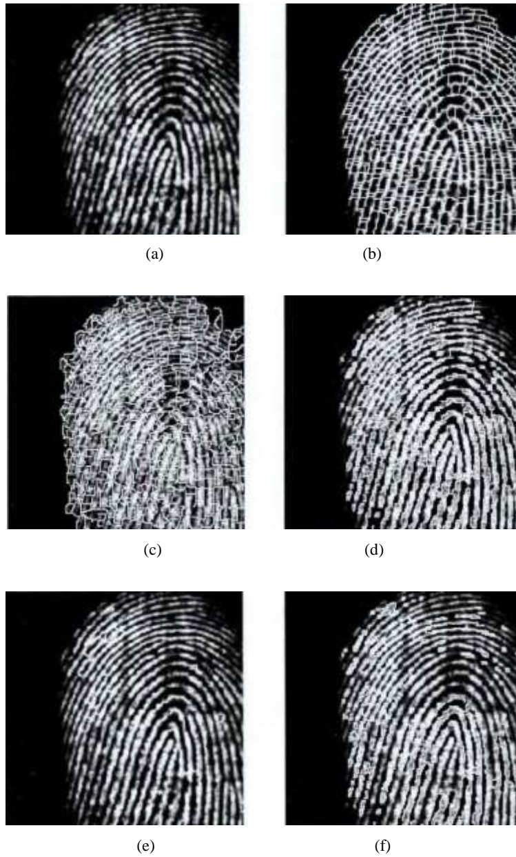
Fig. 3. Results of edge detection obtained with fingerprint image: Origin image (a); result of watershed algorithm (b); result of MGA algorithm (c); result of W algorithm (d); result of WT algorithm (e); result of new algorithm (f)
