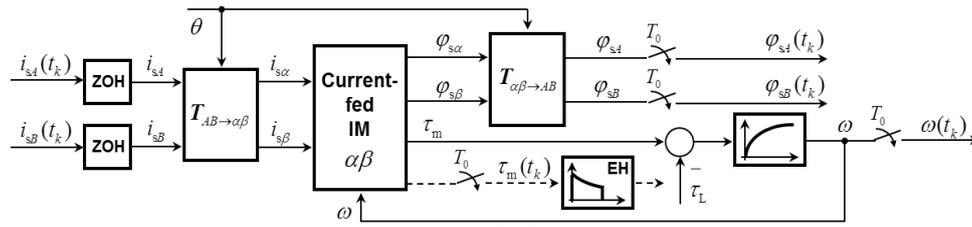
Fig. 1. Discretization scheme
