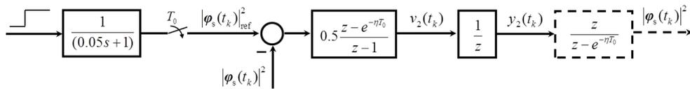
Fig. 5. Outer control loop configuration
