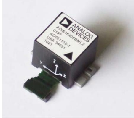
Fig. 1. Inertial Measurement Unit ADIS16405
