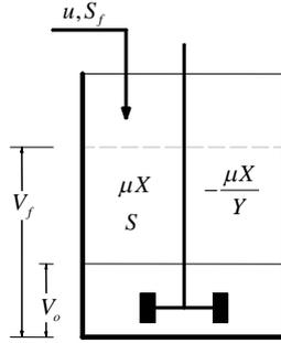
Fig. 3. Sketch of the fed-batch bioreactor of the fermentation process of *Bt*
