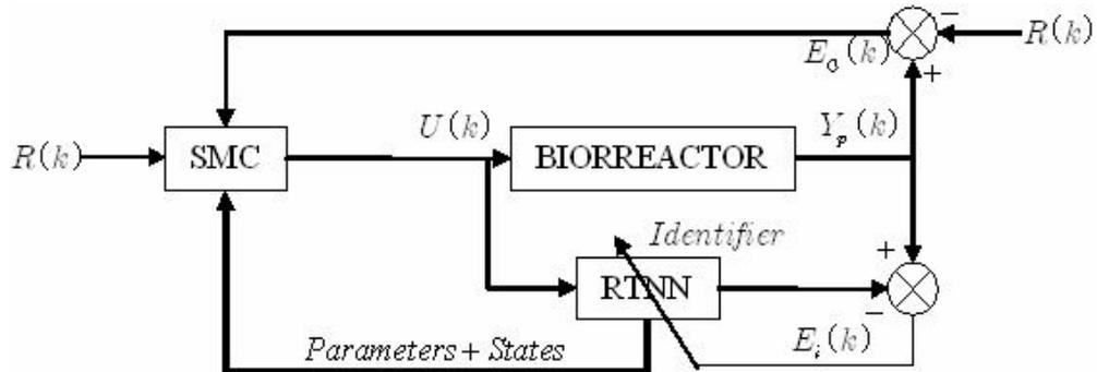
Fig. 1. Block-diagram of the closed-loop system containing neural identifier and sliding mode controller
