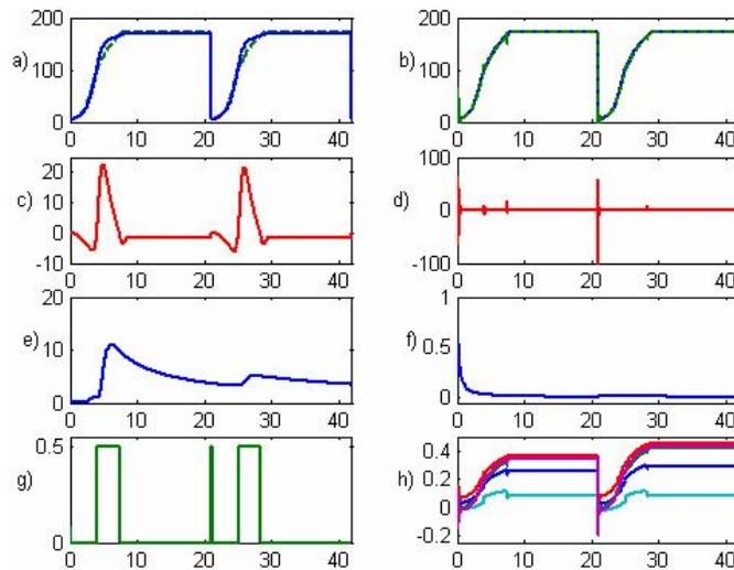
Fig. 4. Simulation results of the discrete-time adaptive SMC of a fed-batch fermentation process: a) comparison of the reference signal with the plant output; b) comparison of the output of the plant with the output of the identification RTNN; c) instantaneous error of control; d) instantaneous error of identification; e) mean square error of control; f) Mean square error of identification; g) control signal; h) systems states, estimated by the identification RTNN
