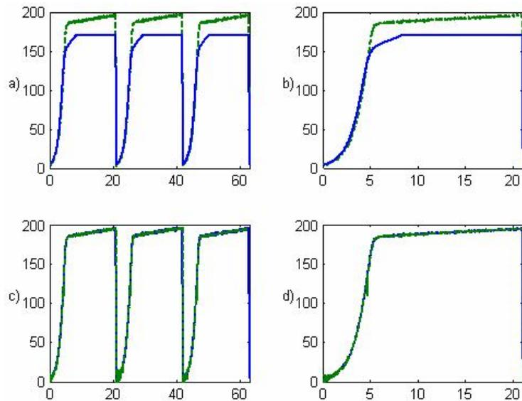
Fig. 7. Simulation results of the discrete-time adaptive SMC without  $I$ -term and with 10% constant process noise, applied for a fed-batch fermentation process; a) comparison of the reference signal with the plant output for three cycles; b) detailed view of a) for one cycle; c) comparison of the output of the plant with the output of the identification RTNN; d) detailed view of b) for one cycle
