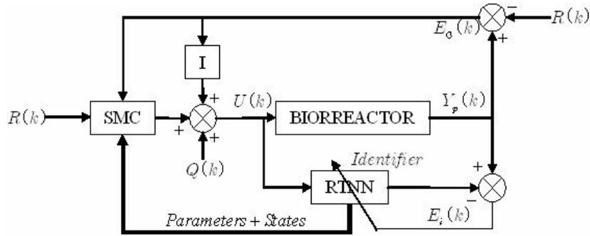
Fig. 2. Block-diagram of the adaptive SMC system, with a neural identifier and an  $I$ -action
