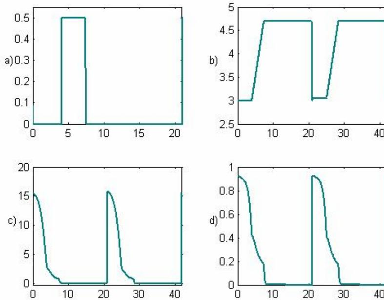
Fig. 5. Additional simulation results of the discrete-time adaptive sliding mode control application: a) control signal; b) evolution of the culture volume into the bioreactor; c) evolution of the limiting substrate in the bioreactor; d) evolution of the specific growth rate  $\mu(S(t))$
