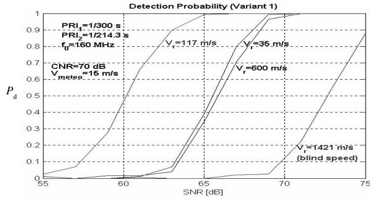
Fig. 7. Variant 1 – detection probabilities in the case of moving clutter
