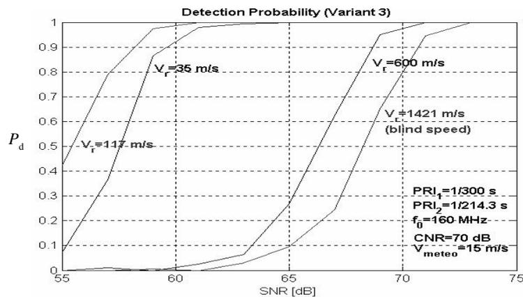
Fig. 9. Variant 3 – detection probabilities in the case of moving clutter
