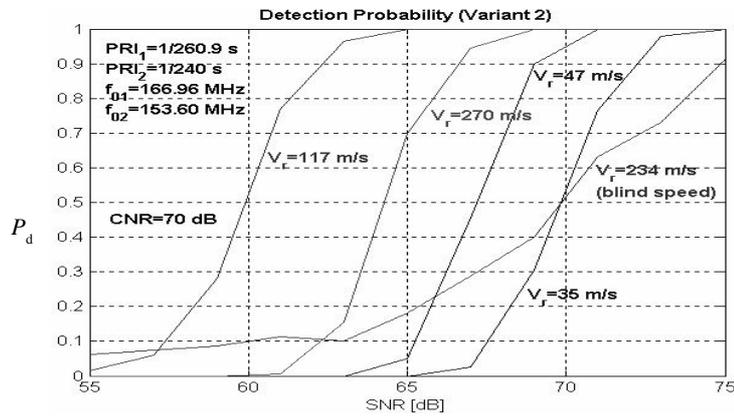
Fig. 5. Variant 2 – detection probabilities in the case of unmoving clutter
