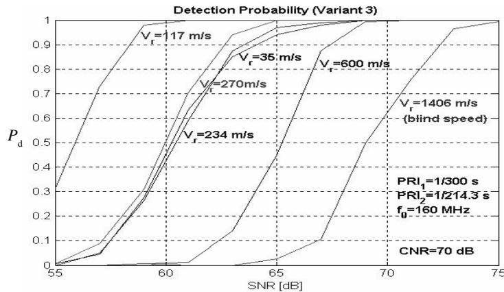
Fig. 6. Variant 3 – detection probabilities in the case of unmoving clutter
