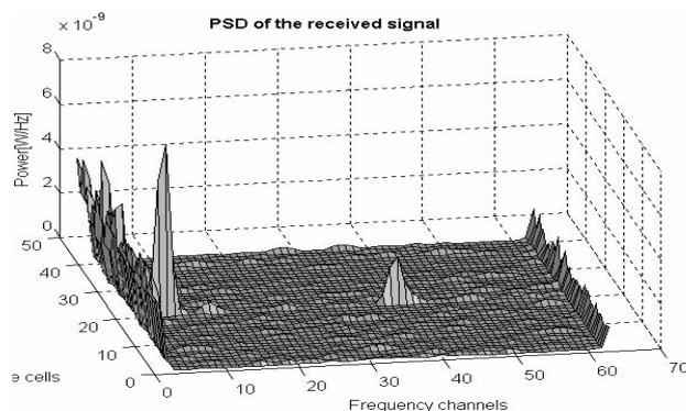
Fig. 3. Variant 3 – power spectral density of the train's returns
