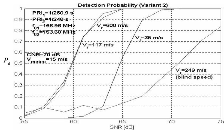
Fig. 8. Variant 2 – detection probabilities in the case of moving clutter
