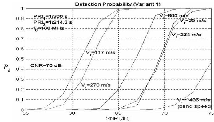
Fig. 4. Variant 1 – detection probabilities in the case of unmoving clutter
