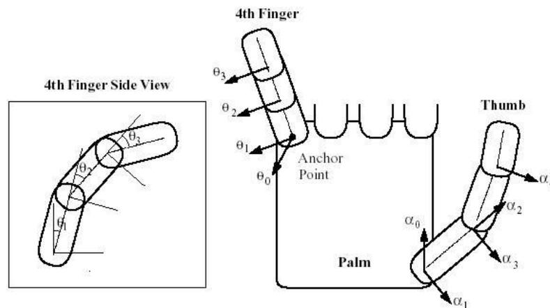
Fig. 4. Kinematic models, illustrated for forth finger and thumb [25]
