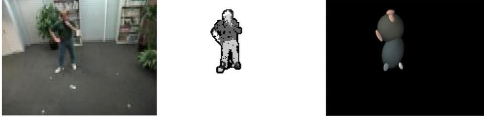
Fig. 1. Video input (left), segmentation (center) and 2D representation of the blob statistics (right) [30]
