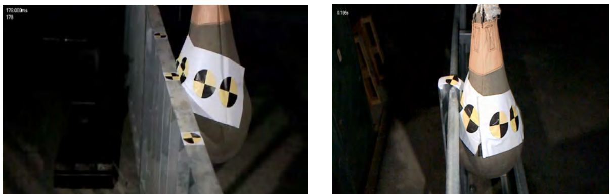
Figure 10. Strike between soft elastic body and pedestrian railing
